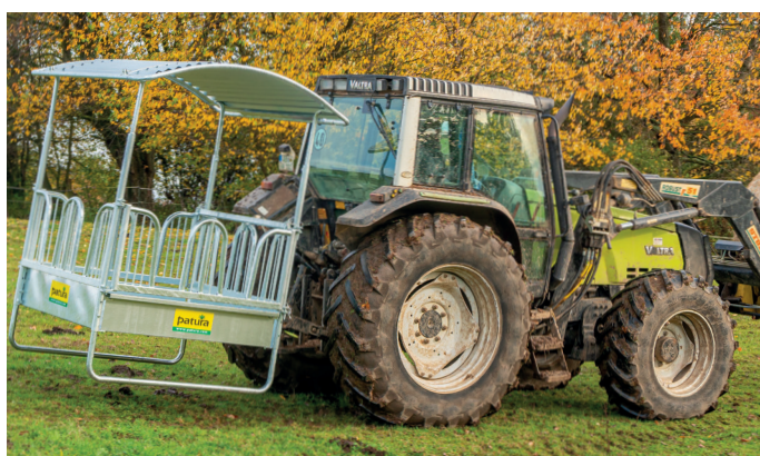
Transport using a 3-point linkage, up to 10 km/h when empty
